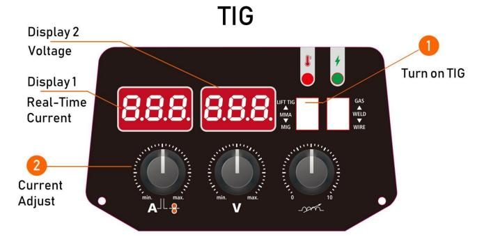
Display 1:Real-time Current, Only displayed during TIG welding
